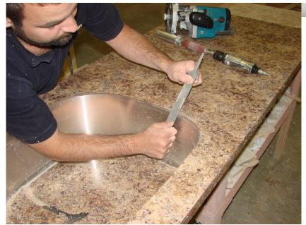
Removal of the last remaining overhang of laminate and seaming adhesive may be accomplished by hand filing. Use an assortment of files including flat, round or half moon files to hand file the edge of the laminate until it is flush to the bowl wall.
