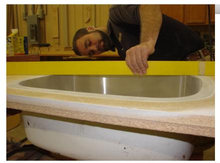
Check for level (low or high spots) after sanding has been completed. Make sure the inside wall of stainless steel sink is not raised. Ensuring a flat and level substrate and sink is important for a quality installation.
