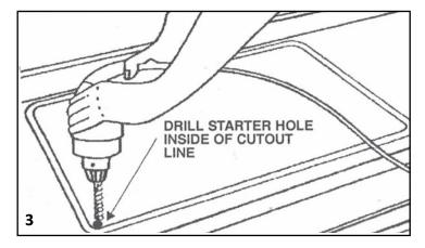
Drill a starter hole just inside of the cut line.
