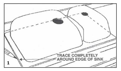
If a paper template has been provided, follow the instructions on the template. If no template is available, use the sink as your template. Place sink upside down in the position where sink is to be installed. Pay attention to backsplash and sink cabinet constraints such as tip-out trays. Trace around the sink.
