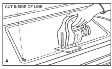
Use a jigsaw to make the cutout. If you are using a countertop material other than laminate, you will need to use the appropriate router and hard surface template to accomplish the cutout.
