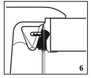
Attach supplied clips to the anchor points on the underside of the sink rim. Styles of clips may vary by sink type. Place a bead of a good quality silicone on the underside rim of the sink. Locate the sink correctly in the cutout in the countertop and tighten the sink clips. Wipe up excess silicone with a damp cloth.
