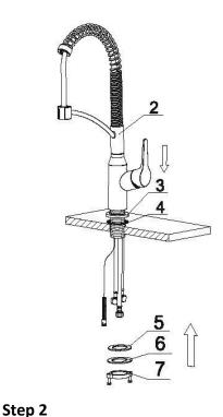
Insert the main body into hole with the base (3) and rubber washer (4). Re-install the rubber washer (5), metal washer (6) and mounting hardware (7) from the bottom.
