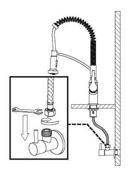
**Step 6**Connect the water lines to the outlets tightly. Turn on the outlets and check for leaks.
