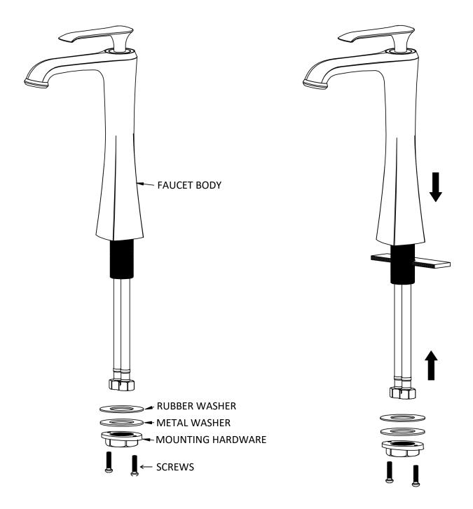
**Step 1**Remove rubber washer, metal washer and mounting hardware from faucet body.
