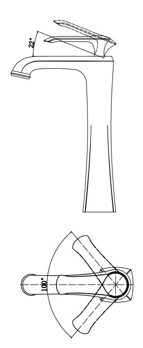
Lift the handle lever upward to turn the water on.
