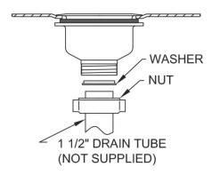
MAKE SURE WASHER IS IN POSITION, SLIDE NUT ON 1-1/2" DRAIN TUBE. PUSH TUBE INTO DRAIN BODY AND HAND TIGHTEN NUT. TEST FOR LEAKS.
