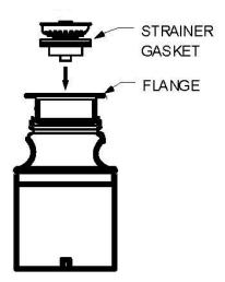
LUBRICATE GASKET ON STRAINER WITH WATER AND PUSH SLOWLY INTO THE FLANGE.
