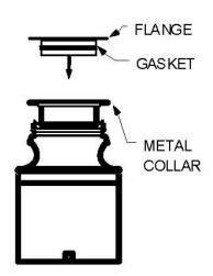
LUBRICATE FLANGE GASKET WITH WATER AND PUSH FLANGE SLOWLY INTO METAL COLLAR.
