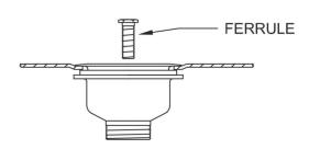
LINE UP RIBS IN DRAIN BODY AND STRAINER FLANGE THEN SCREW IN FERRULE. CAUTION: HAND TIGHTEN THEN 1/4 TURN WITH SCREWDRIVER. DO NOT OVER-TIGHTEN.
