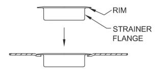
APPLY A NON-ACID SILICONE UNDER THE RIM OF THE STRAINER FLANGE AND PUSH DOWN INTO SINK.
