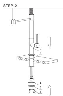
2. Insert the main body into the hole with the "O" ring(3), refix the rubber washer(4), metal washer(5), mounting hardware(6) from the bottom.
