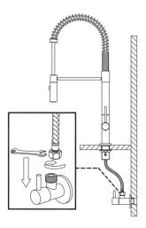
4. Connect the waterlines to outlet tightly. Turn on the outlet and check for leaks.
