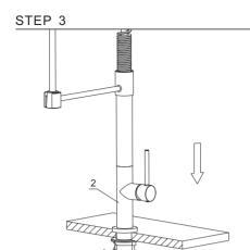
3. After adjusting the direction of the main body(2), tighten the mounting hardware (6) with hands and tighten the screws(7) with a Philips screwdriver.
