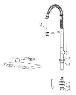
Remove the mounting hardware(6), metal washer(5), rubber washer(4) from the main body(2);
